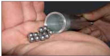
Pull the pounder out the holder and fill in the steel balls (not more than 12).
