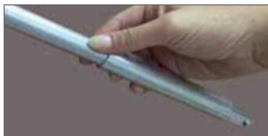
Insert the pounder carefully and the tool is ready for use. If too much pressure is applied, the balls are pressed out at the bottom at the tool. Handle with care!
