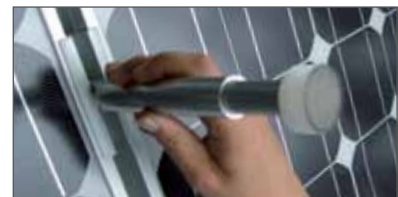
Hammer in the ball using a plastic hammer . The head of the pounder is made of aluminum and thus is not suitable for steel hammer operations.
