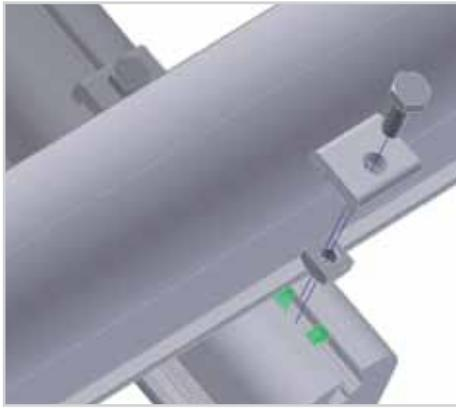
Image 1 Fastening of the lower mounting rail
